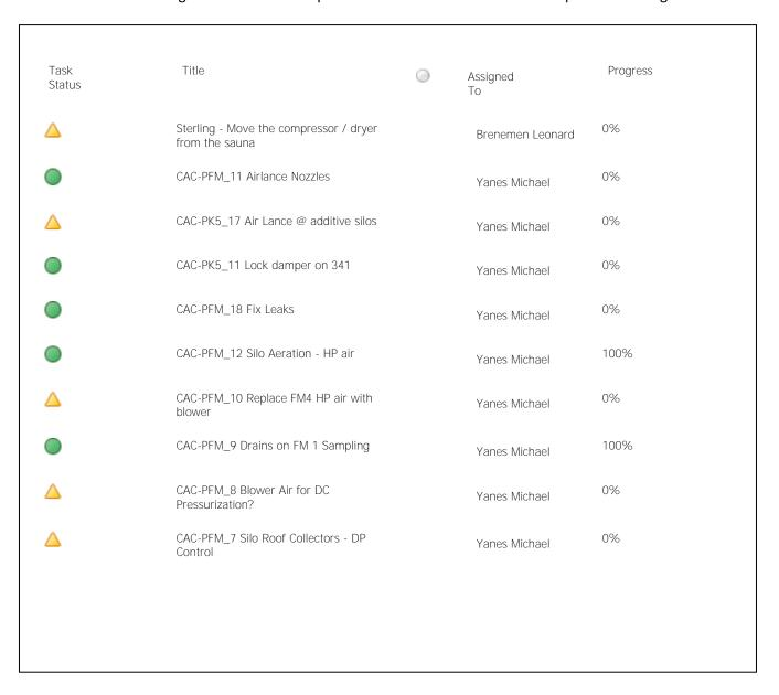
➤ Dust Collector Optimization tracking tool on SharePoint – All Dust collectors in Titan were documented here along with name plate data. As plants complete conversion to more energy efficient Differential Pressure control and Regulate incoming compressed air lines to the lowest possible setting – the changes are recorded to show Titan America progress and help estimate initiative savings for management progress reports. This communication drives performance.
