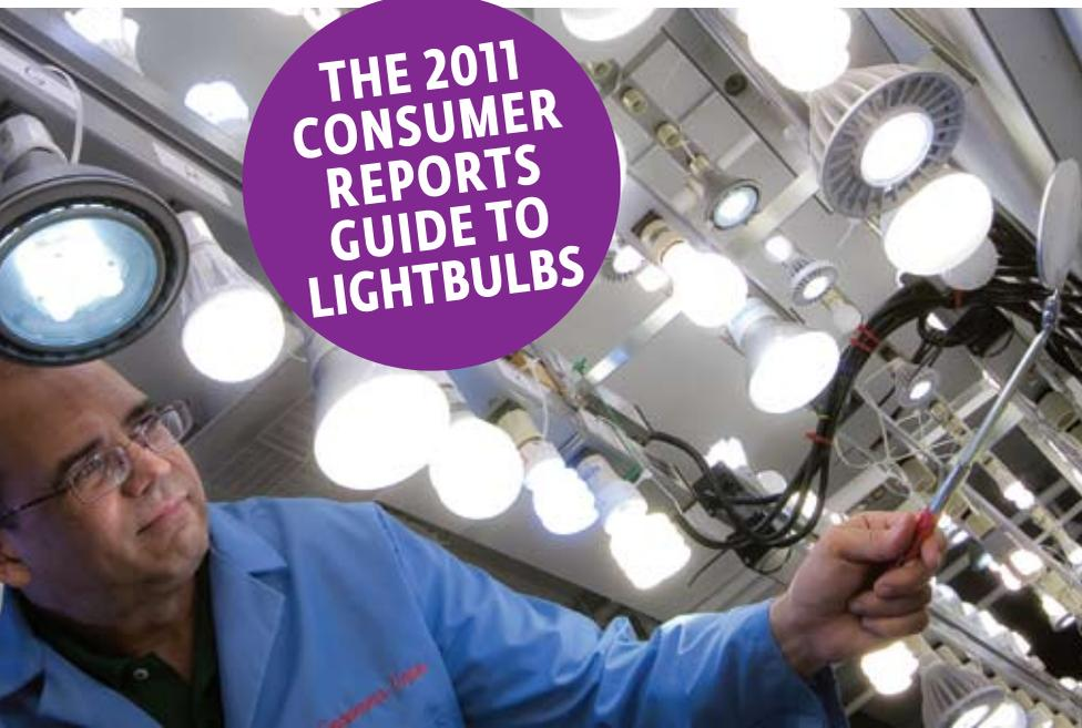
**POWER TRIP** We run each bulb through on-and-off cycles to rate its brightness and durability.
